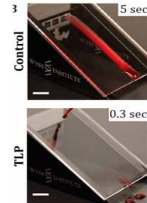
A drop of human blood adheres to uncoated acrylic (top) but is repelled by TLP coated acrylic (bottom) (Scale bar 1cm). Leslie et al. 2014.
