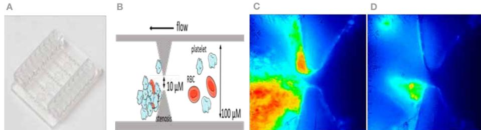
Microfluidic devices for measuring thrombotic and bleeding tendency. (A) Biochip containing channels for perfusion of blood. (B) Schematic of a 90% stenosed channel for the study of thrombus formation. (C) Blood sample with increased thrombus formation. (D) Decreased thrombus formation at the stenosis site.
